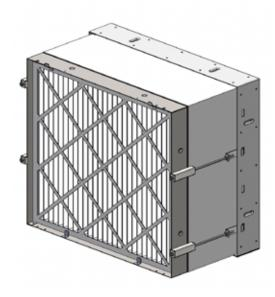
**Application:** The RFHA Series is a combination of two styles of filter frames to provide a modular two-stage filtration system. The RFH HEPA Holding Frame that is designed to hold a gasketed HEPA filter is connected via the HEPA clamp to RFA Universal Holding Frame designed to hold a 2" pleated pre-filter. This combination two-stage modular frame system can be part of a built-up filter bank on the jobsite or in OEM factory-produced air handling units.
